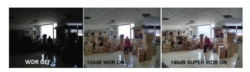
reproduction even under the extreme back light and high contrast conditions. The ratio that the brightest light signal values divided by the darkest light signal values is up to 140dB.
