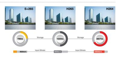
S+265 can save approximate 50% bitrate than H.265 technology, saves 70%-80% bandwidth compared with H.264
