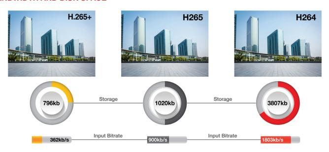
H.265+ can save approximate 50% bitrate than H.265 technology, saves 70%-80% bandwidth compared with H.264
